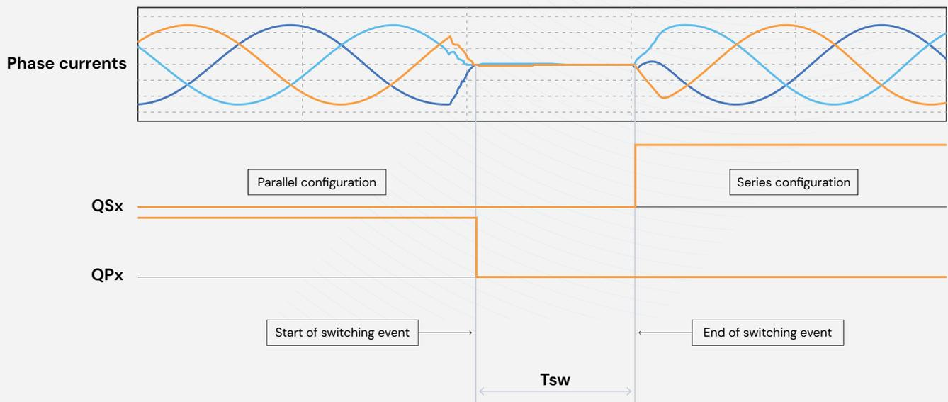
Figure 1. Traditional switching sequence, parallel to series.
