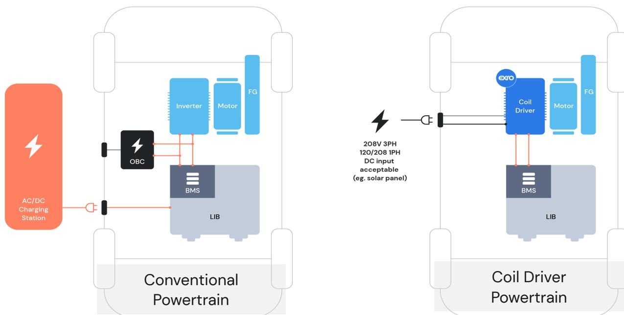
**Figure 2. The drawings are to illustrate how Exro’s Coil Driver™ technology new feature can eliminate the need for onboard OBC or external charging infrastructure.<sup>3</sup>**
